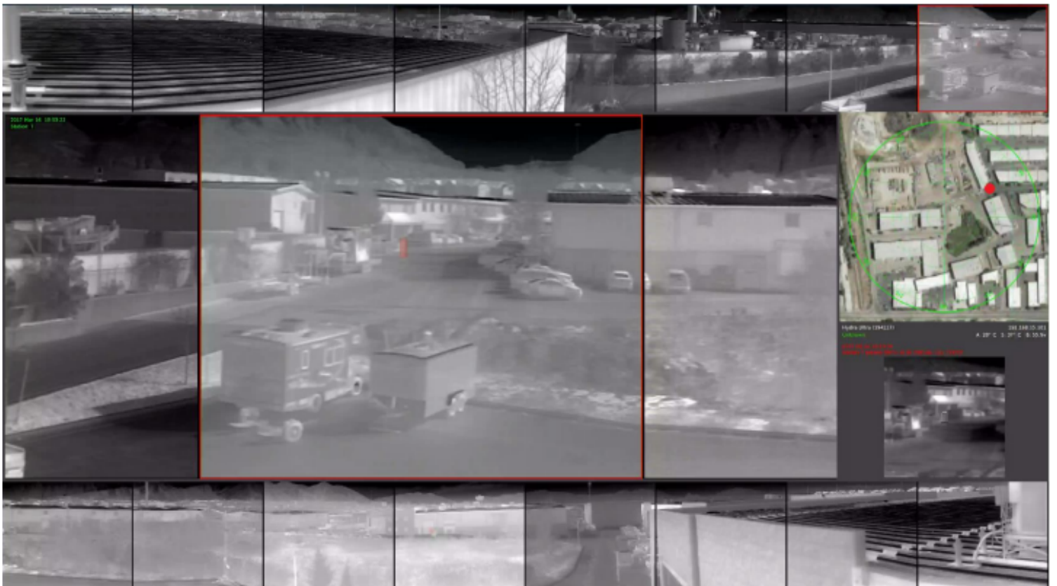
Figure 2. Thermal Radar 360° RTSP (180° FOV on Top, 180° FOV on Bottom, Geospatial Map, Zoomed Alarm Window)
